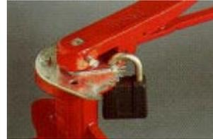
**Padlock Kit** allows the customer to lock the valve in the full open or closed position, tamper proofing the valve. By drilling a new hole in the top plate, the handle can be locked in mid travel.
