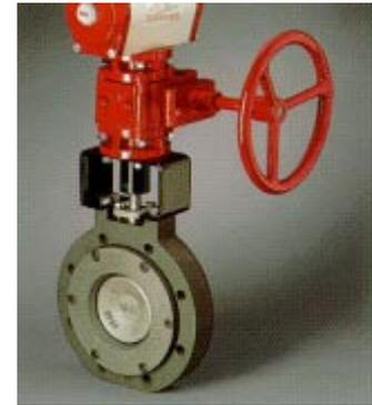
**Operation** Any residual air pressure in the pneumatic actuator must be vented before operation of the Declutchable Gear Operator. Bray recommends the use of a vent valve to block the incoming air supply and vent residual air. Then engage the declutching lever and rotate the valve using the handwheel. When returning to automatic operation, disengage the manual override by rotating the declutching lever, turning the vent valve to off, then restoring air pressure to the actuator.
