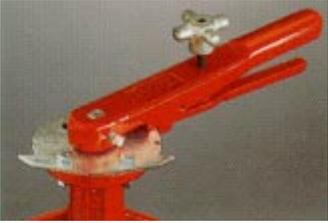
**Infinite Position Notch Plate** for throttling applications, allows for very precise adjustments of valve disc positioning anywhere from 0° to 90°. Positioning is simply a matter of loosening the set knob, moving the handle, then retightening the knob. *For resilient seated valves only.*
