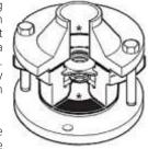
The 'cam' design of the body allows the various flange types to be accommodated. The body is rotated to touch the flange joint bolts ensuring that the valve is centered in the pipeline.
